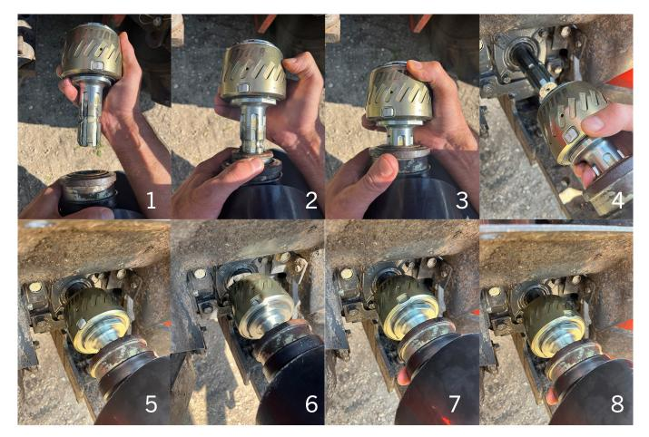
Bullet PTO coupler adapter connection method Guide - **for tractors with free spinning PTO shaft**. Read your owners manual in additon to using this guide.
